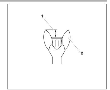
Fig. 13 Correct pilot flame setting
