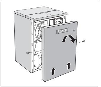
Fig. 1 Removing front panel of boiler
