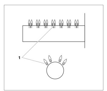
Fig. 14 Main burner **1** Main burner flame
