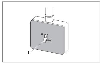
Fig. 10 Switching on heating system (with aquasmart)1 ON/OFF switch (main switch)
