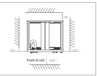
Figure 2 Clearance - top view (including air duct)
