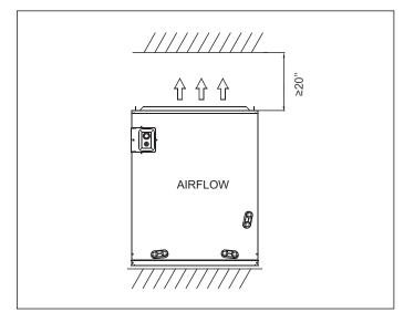
Figure 1 Clearance -front view (including air duct)
