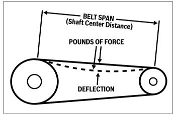
Figure 15 Fan Belt Tensioning
