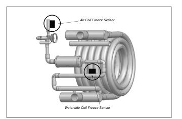
Figure 10 MC Freeze Sensor Locations
