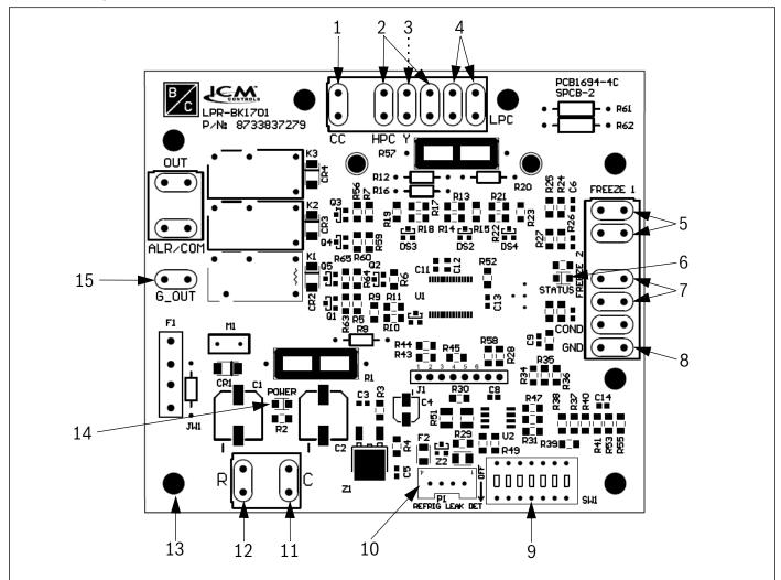
Figure 9 Second-Stage UPM Controller Board
