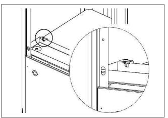
Figure 11 Condensate Overflow Protection Sensor
