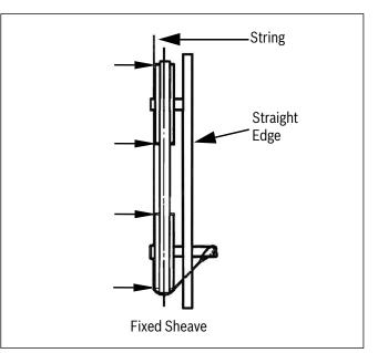
Figure 14 Sheave Alignment
