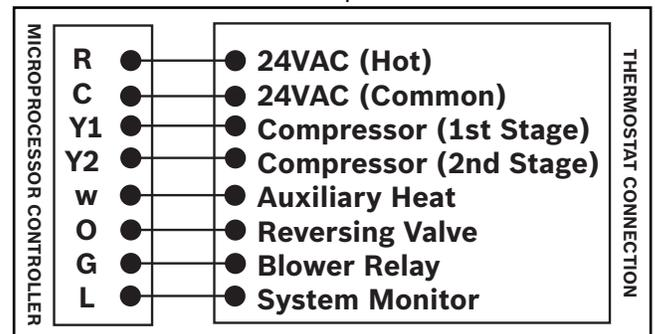
Figure # 15 Thermostat Wiring
