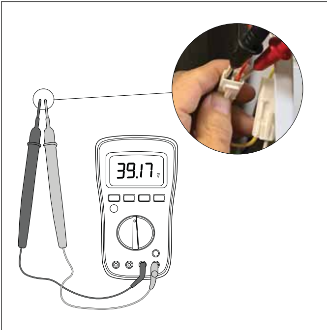
Figure 8 Applied Voltage Measurement Method
