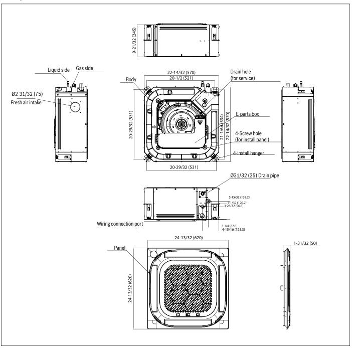
Figure 1 Dimensions in inches (mm)
