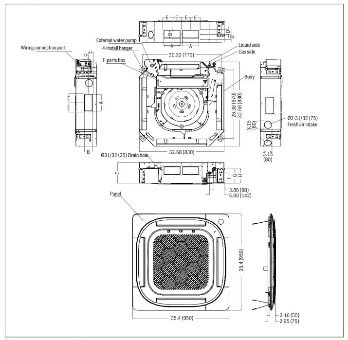
Figure 2 Dimensions in inches (mm)
