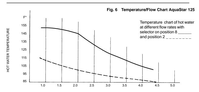
FLOWS IN GALLONS PER MINUTE -based on ground water temperature of 55°F \*Range described above will be lower if inlet temperature is below 55°F
