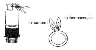
Fig. 4 Characteristic Pilot Flame
