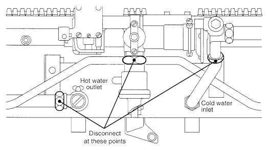
Fig. 3 To Disconnect Heater From Wall Hanging Strip
