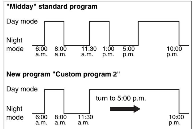
Fig. 11 Linking heating phases
