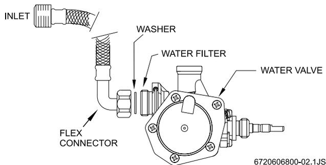
Fig. 6 - Water valve - top view
