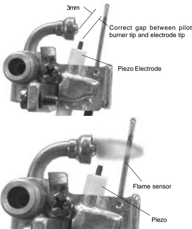
**Fig. 10 - Characteristic Pilot Flame**
