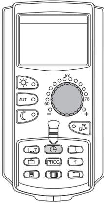
A heating phase consists of two set points – a start and a stop point. To connect two consecutive heating phases, place the stop point of the first heating phase onto the start point of the next phase.
