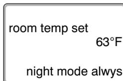
The LED of the night mode button lights up. Now your heating system is in constant night mode (setback heating mode), and operates at a lower room temperature.
