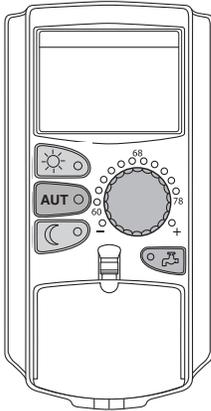
With the flap closed you can adjust the room temperature with the dial. With the flap open, also press "Day mode" or "Night mode".
