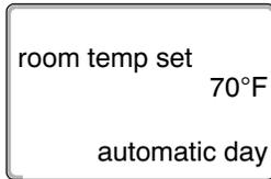
Press and hold down "Temp". First, the heating zone whose temperature you want to adjust is displayed. After approximately 2 seconds, the display will show the currently-selected temperature and operating mode.
