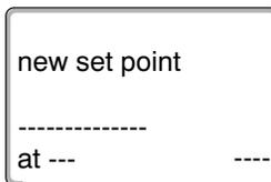
Only after all three details (day/time/temperature) have been set for the new set point will it be automatically saved under "custom program" and the heating zone number (here: "2"). The saving process is not shown on the display. The display shows the blank mask "new set point" for the next set point.
