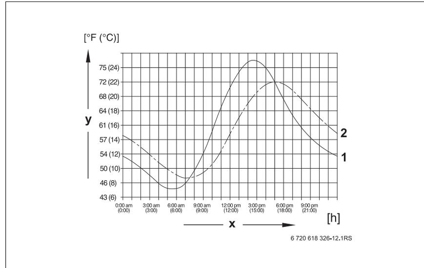
Fig. 15 Current and adjusted outdoor temperatures compared
