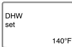
Release the DHW button. The newly-selected DHW temperature is saved within approximately 2 seconds. The permanent display will then appear again.
