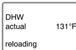
Depending on the size of the storage tank and the boiler output, DHW will be available after approximately 10 to 30 minutes. With instantaneous water heaters or combination boilers, DHW is available almost immediately.
