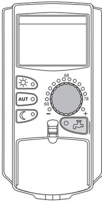
The user interface also offers you the option of heating DHW in an energy-conscious manner. For this purpose, DHW heating can be selected via a timer. You can select between the set values for DHW and "OFF", to stop DHW heating.
