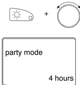
Hold down "Day mode", and **simultaneously open the cover of the MEC2**. "party mode" is enabled. Hold down "Day mode", and turn the dial until the desired number of hours is displayed (here: "4").
