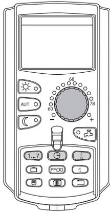
You may enter up to 42 set points per week and heating zone to create a new heating program. A single set point comprises three details: weekday, time and temperature.
