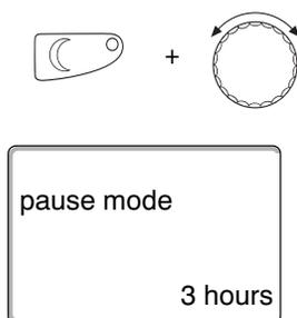
Hold down "Night mode", and **simultaneously open the cover of the MEC2**. The "pause mode" is enabled. Continue to hold down "Night mode", and select the desired (here: "3").
