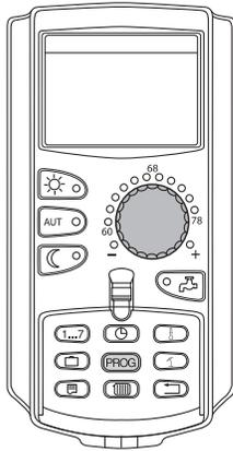
The MEC2 remote control is equipped with eight different, preset heating programs that act as standard programs. See the following page for a summary of the preset times of the standard programs.
