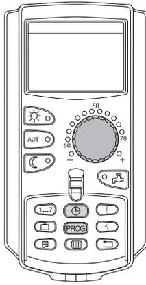
If the set points, i.e. the times of a standard program when the system changes over between day and night mode, only partially suit you, you may change them, or ask your heating contractor to change them for you. The modified standard program is saved under "custom" and the number of the heating zone. The heating program memory is available for this.
