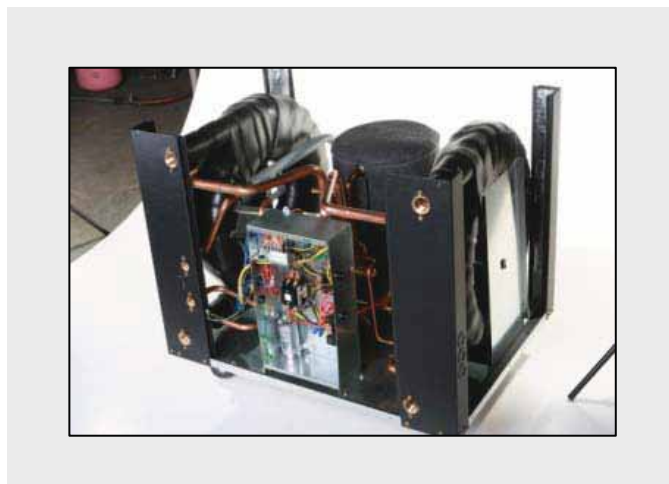
Fig. 11 Water to water heat pump internal view
