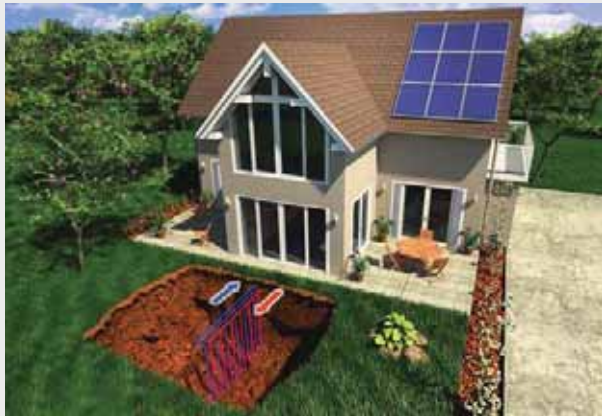
Fig. 30 Closed loop vertical design
