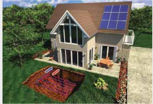
Fig. 31 Closed loop horizontal design
