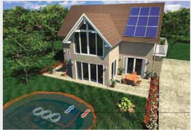
Fig. 32 Closed loop pond or lake design
