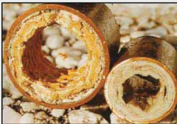
Fig. 22 Scaling Courtesy of International Ground Source Heat Pump Association/Oklahoma State University
