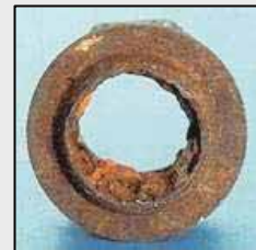
Fig. 23 Encrustation Courtesy of International Ground Source Heat Pump Association/Oklahoma State University
