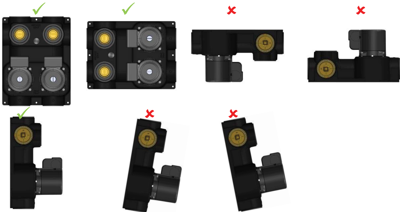
Figure 2: Acceptable mounting positions for Flow-Link™ series flow centers
