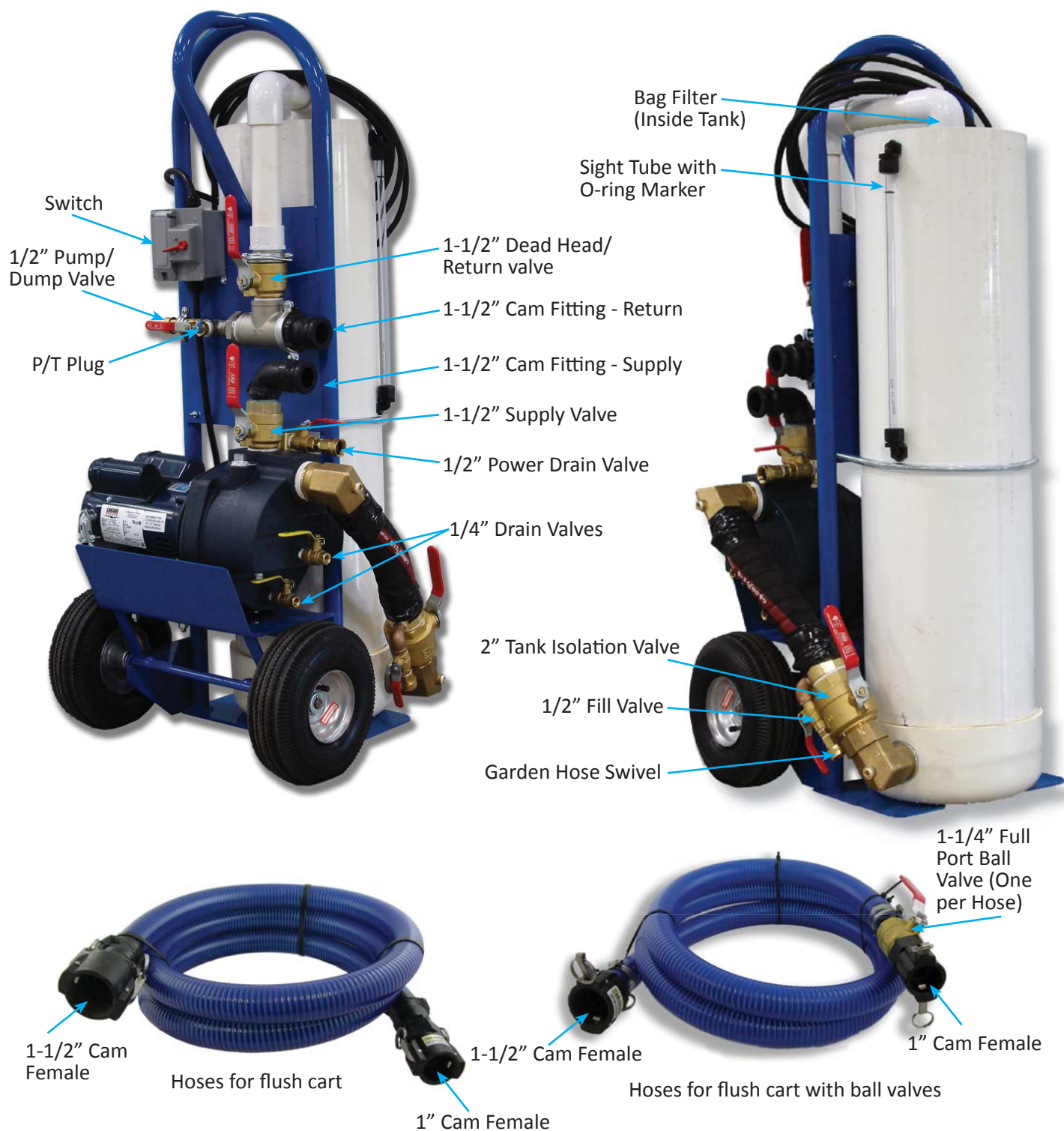
Figure 9: Flush cart diagram with descriptions
