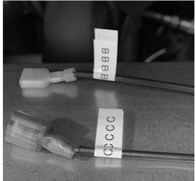
Fig. 19 Leave B and C Disconnected
