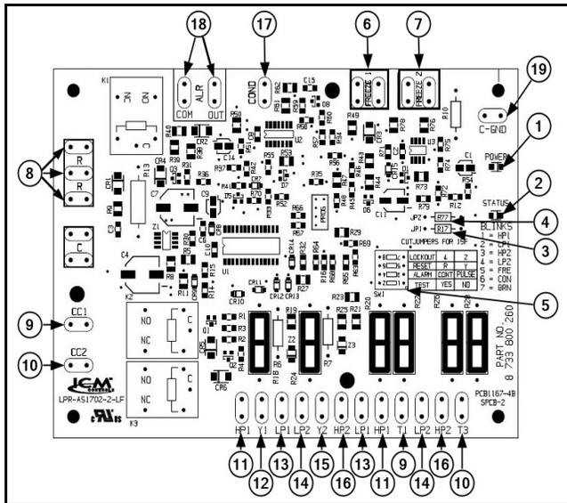
Fig. 11 UPM II controller board
