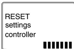
The blocks in the last line disappear one after another. The reset occurs when all blocks have disappeared. If the button is released while a block is still visible, the reset is canceled. After implementing a reset, the display automatically reverts to the next level up.
