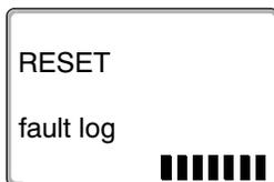
The blocks in the last line disappear one after another. The service call is reset after the final block has disappeared. Reset will be terminated if you release the button before all blocks have disappeared. After implementing a reset, the display automatically reverts to the next level up.
