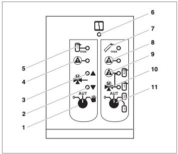
Fig. 1 Front panel of FM443 function module
