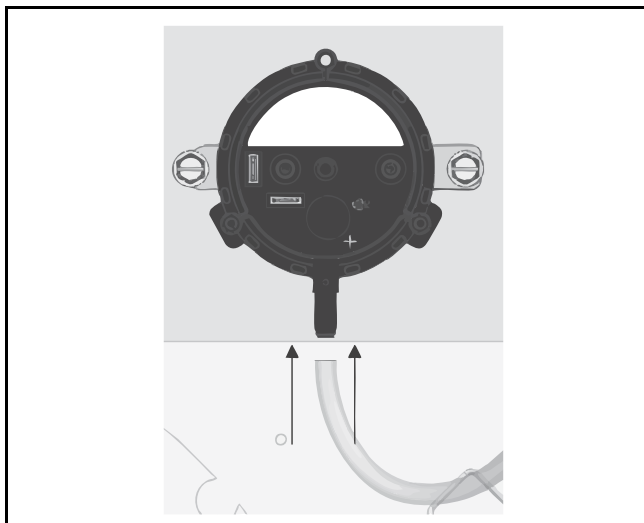
Fig. 16 Connect Tube to the APS Vacuum Port
