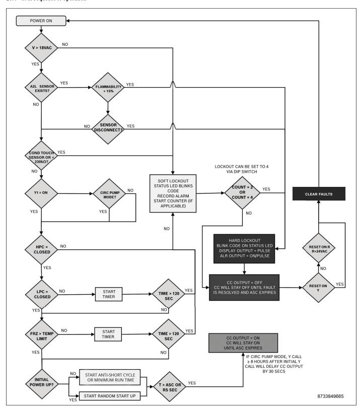
Figure 11 UPM Sequence of Operation Flowchart
