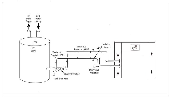
Figure 13 HRP System Setup
