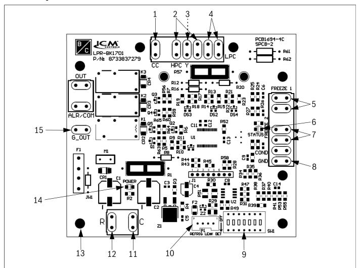
Figure 8 Second-Stage UPM Controller Board
