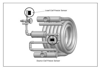
Figure 9 Source Coil Freeze Protection Sensor (FREEZE 1) and Load Coil Freeze Protection Sensor (FREEZE 2).
