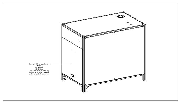
Figure 21 Service Clearance, TW122
