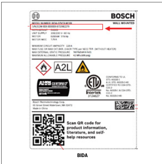
Figure 32 BIDA indoor unit rating plate
